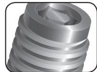
Coarse thread (example: aluminum 425 g/60 L CO2 cylinders of Limo Bar brand)
